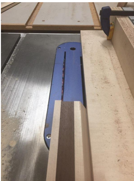
Photo 5 - setup for initial squaring cut.
