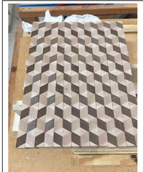
Photo 9 – final strip arrangement after strip flips. The 4 strips on the left are not arranged correctly
