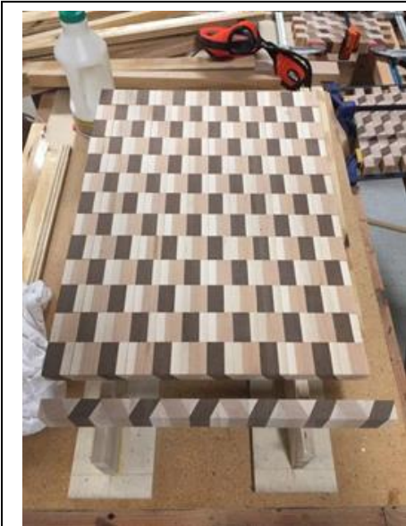
Photo 10 – Strips rotated for final glue up
