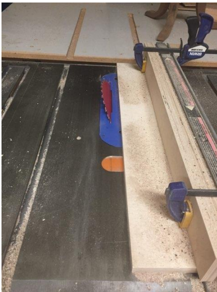
Photo 3 Fence ready to cut the strips
